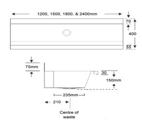
Stainless steel wash troughs supplied with time flow knee operated valves and chrome plated basin spouts.
