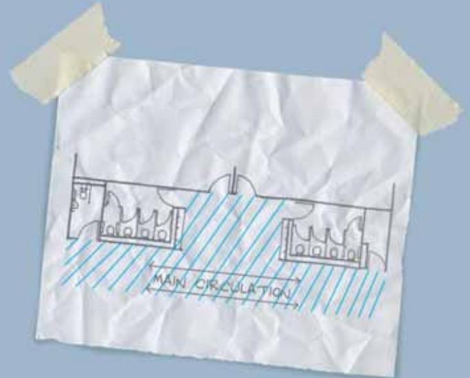
▲ Above hand wash extension of circulation
