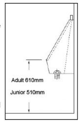
For wall hung and floor standing urinals with fixing holes in the top flange and ends the urinal should be fixed to the wall with appropriate fixings (not supplied).
