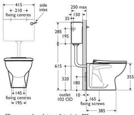
FFL to centre line of cistern fixing holes 890
